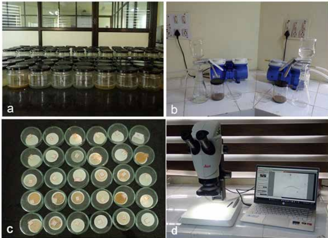
Separation of microplastic techniques- a: Digestion of samples; b: Filtration of digested samples; c: filtrate enclosed in petri dish; d: detecting and sorting microplastics through Leica S9i stereozoom microscope
